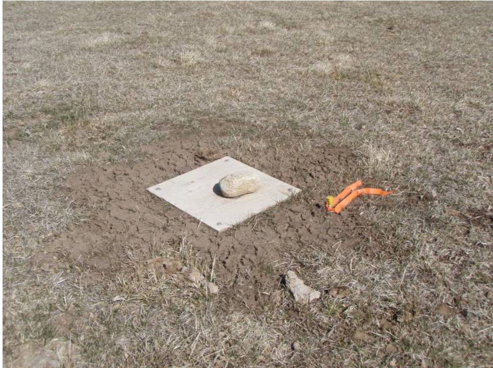
Groundwater monitoring well in floodplain of West Fork Carson River, March 2009
